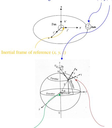
Earth spherical coordinates  $(\lambda, \phi, r)$  Local coordinates (x, y, z)
