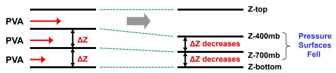
• Hydrostatic balance (and the hypsometric equation) requires ALL changes in thickness ( $\Delta Z$ ) to be accompanied by temperature changes...
