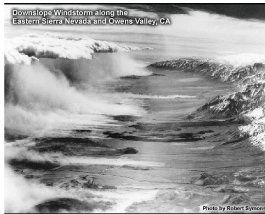
Fig. 3.5: A hydraulic jump in a supercritical airflow over the Sierra Nevada mountain range, made visible by the formation of clouds, and by dust raised from the ground in the turbulent flow behind the jump. (Lin 2007; Photographed by Robert Symons, published in Communication on Pure and Applied Math , 20, no. 2, (review by M. J. Lighthill, @John Wiley and Sons, Inc., 1967).
